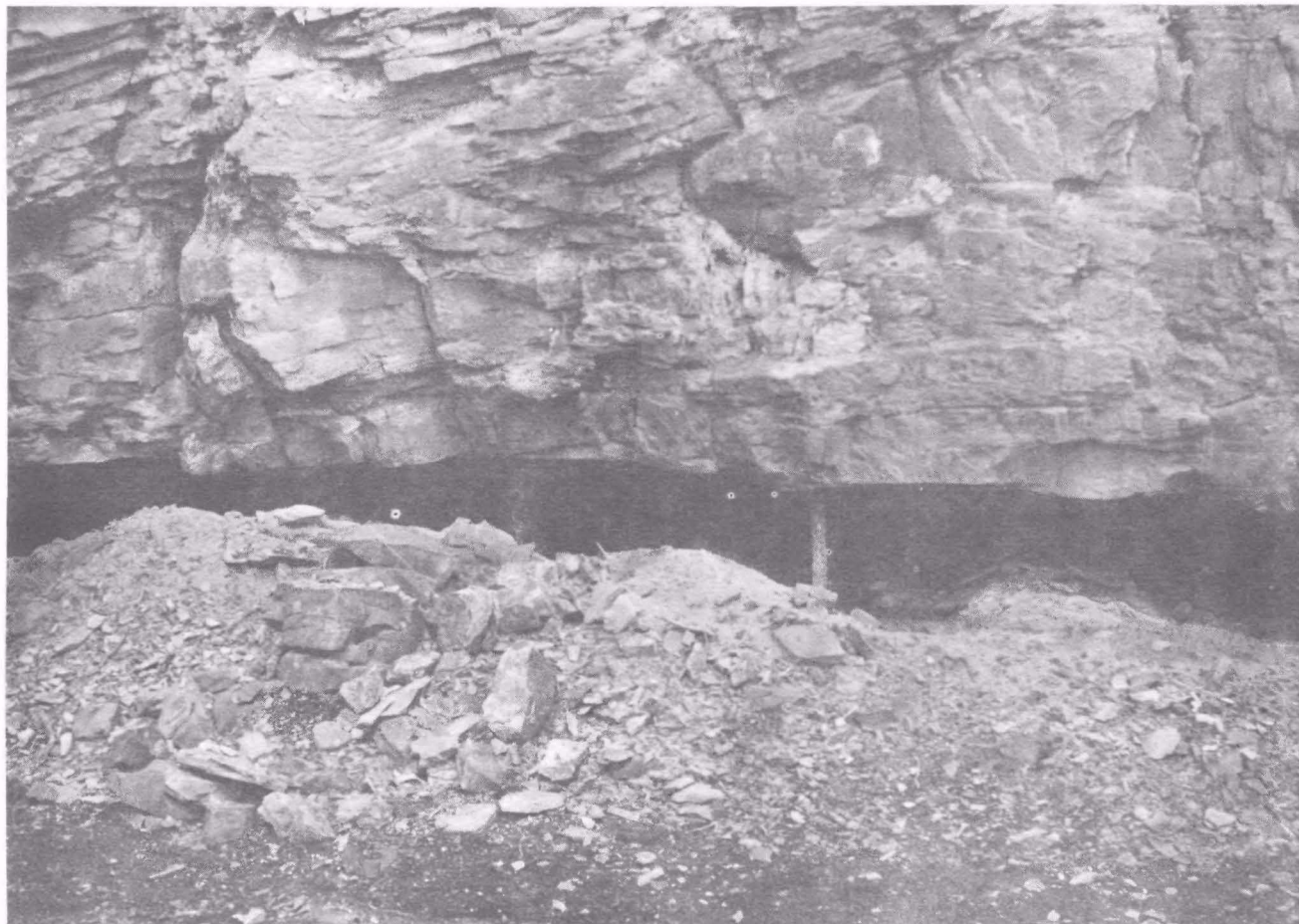
AUGERED AREA ILLUSTRATING EXTENT OF HIGHWALL UNDERMINING SECTION G, STRIP AREA R FIGURE 37
